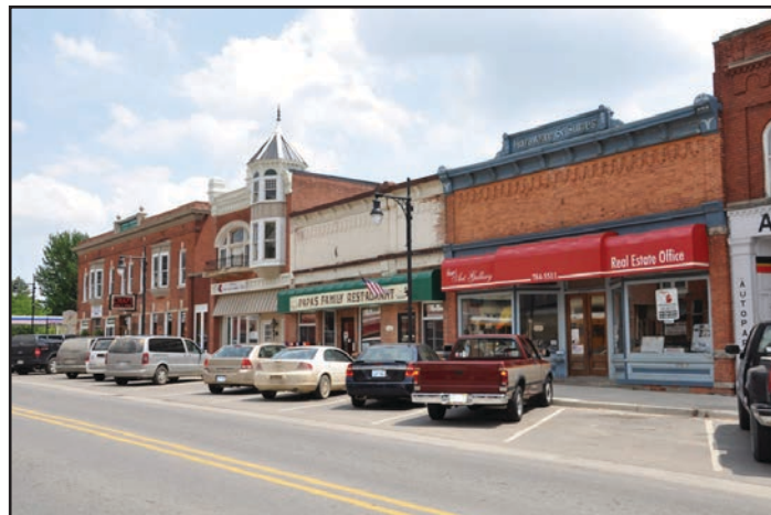
Figure D22: Angled parking provides a barrier between pedestrians on the sidewalk and traffic. The potential that a parked car will back out of a spot also serves to slow traffic on the street.
