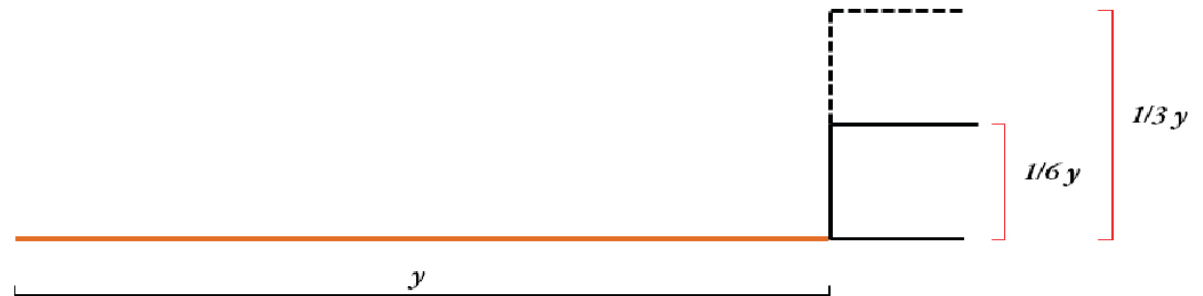
Figure D40: A simple schematic showing the range of building heights deemed appropriate in a Neighbourhood Activity Centre. In this case, ideal building heights range from one-sixth to one-third the width of y , which represents the width of a street (including sidewalk and boulevard), amenity space or both.
