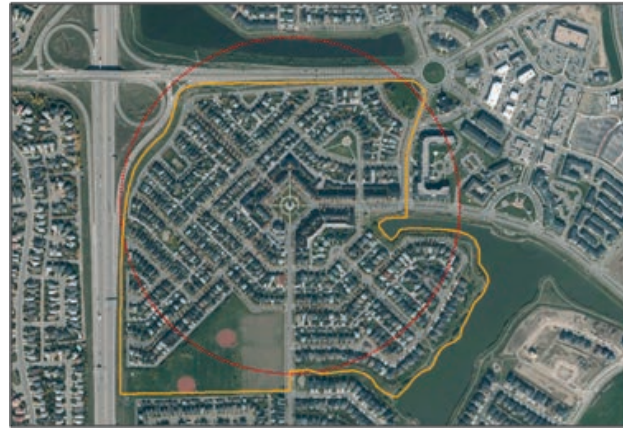
Figure D4: This image shows a neighbourhood with a well-defined edge. The orange line roughly delineates the edge of Inverness, a neighbourhood in southeast Calgary. The edge is composed of an expressway to the west and Arterial streets to the north and northeast. The remainder of the neighbourhood is delineated by school sites (southwest) and linear parks and a small community lake (southeast).
