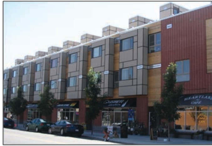
Figure D37: This photo shows a well-designed mixed-use street in Bridgeland. The building provides entryways to businesses at short and regular intervals, creating multiple points of interest for pedestrians. Extensive coverage of windows along the sidewalk also adds to pedestrian comfort by providing “eyes on the street.”
