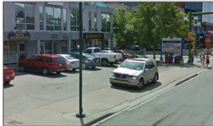
Figure D32: This image demonstrates unacceptable streetscape design further south on the same street: A commercial building with a parking area between the building and sidewalk creates conflict between automobiles and pedestrian movement.
