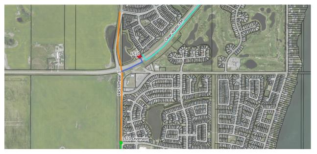
In this servicing stage, LS13 can support 450 L/s or 530 L/s of PWWF depending on the number of pumps installed (approximate service population of 28,200 or 33,600 respectively, derived using the method in Section 4.2) and Lift Station 10 handles flow from an existing population of approximately 14,200 with a PWWF of 223.5 L/s. This represents a total City population of at least 42,400, which is the 25-year build-out population in the existing UMP.
