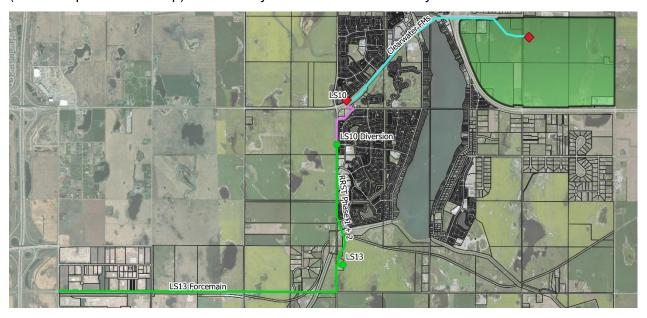
A new lift station in Clearwater Park will discharge into new forcemains that are approximately 3.8 km long which discharge up to 93.5 L/s into LS10 for this servicing stage. It is recommended to stage the construction of the Clearwater Park Lift Station and forcemains to reduce risk of H2S generation associated with long retention time.
